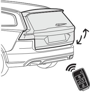
**EN** During installation on a car with automatic tailgate opener, operate the tailgate manually. Sudden and unstoppable movement of the tailgate may cause harm. Check your vehicle owner's manual for more specific information on how the automatic tailgate operates.
